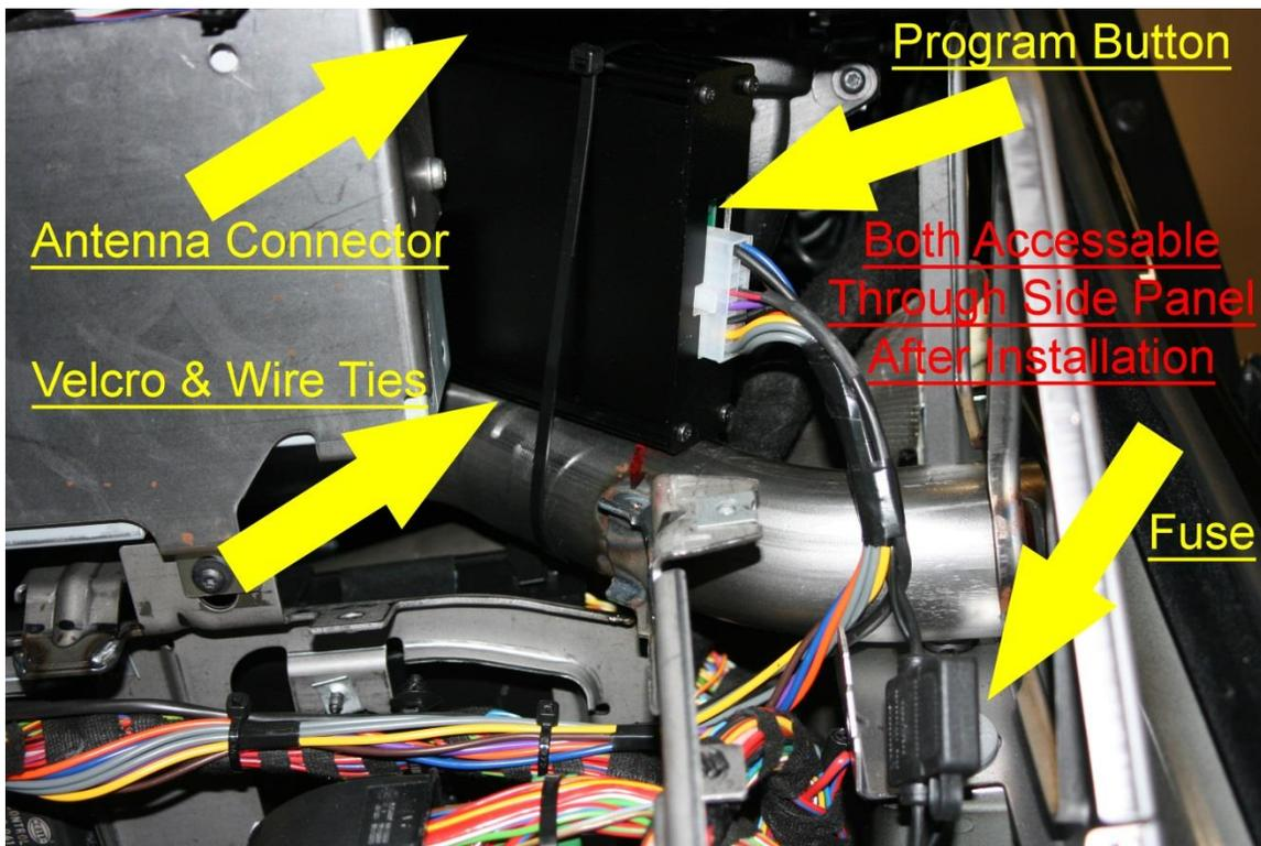
In the kick panel, Ground the **Black Wire to the 10mm Ground Bolt**. Crimp a Yellow T-Tap on the **Red/Green Wire** and plug in the Red Wire:
