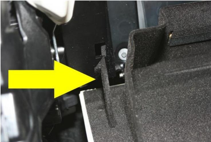
Have on hand, a pointed tool to release two connector tabs:
