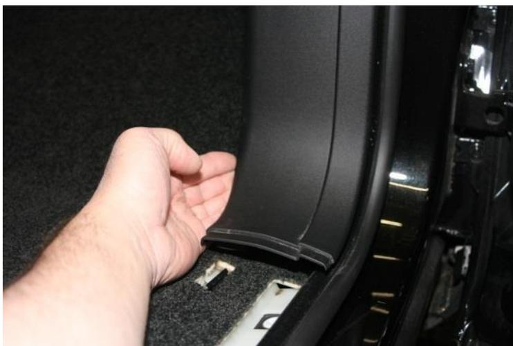
Remove the plastic panel, on the right side of the dash, by prying straight out:
