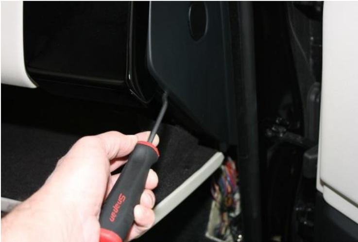
Remove the lower foot well panel held by 3 T20 Torx Screws and unplug the light:
