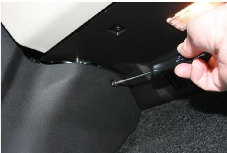
From the rear, bottom edge, pull OUT and DOWN to remove:
