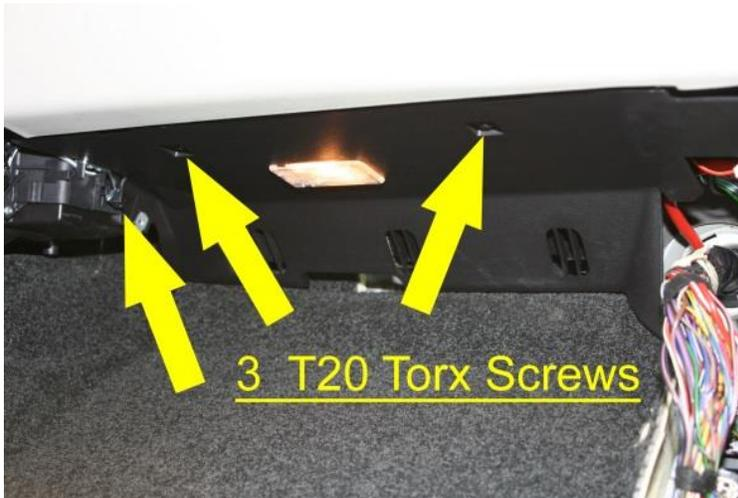
Unplug the 3-Pin connector under the right side of the lower glove compartment and remove the "9<sup>th</sup> T20 Torx Screw" while you're there:
